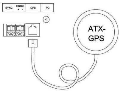
When attaching wires to the terminal block the ATX6 should be in a vertical position. If the ATX6 is horizontal the terminal block will not lock down the wires.
